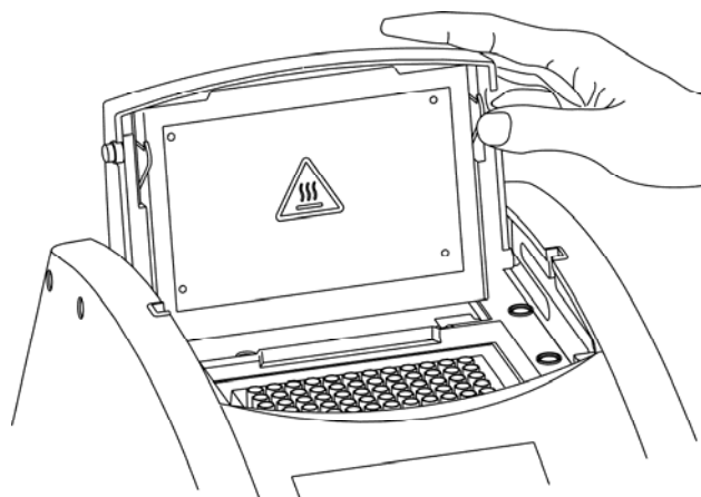
Figure 8. Rest the lid in vertical position
