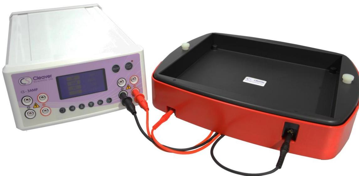
12. Attach the power leads to the appropriate sockets, red to red, black to black on a power supply. **Do not invert the leads or connect up incorrectly as this will cause corrosion of the stainless steel electrode.**
