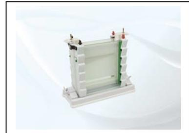
8. Transfer the PAGE insert to the gel tank. Fill the inner and outer buffer chambers before loading samples.
