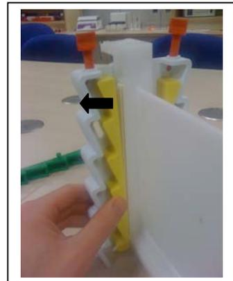
6. Withdraw the sliding gel clamps so that they sit suspended in the resting slots as shown. Repeat steps 1-6 to replace the remaining green sliding gel clamps. Once complete the PAGE insert is ready
