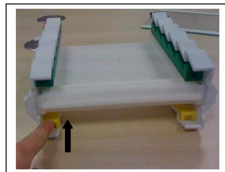
2. Form a 2-gel sandwich on an even bench surface, as described in **General Rules** on page 12 in the Vertical Gel Casting Section. Push the 2-gel sandwich with the
