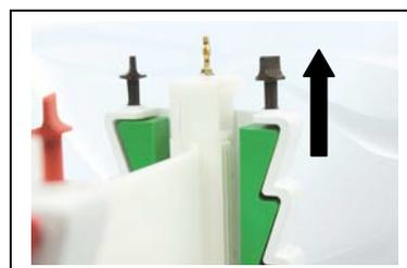
3. Insert a gel cassette into each side of the inner buffer chamber in the PAGE insert, and begin tightening the vertical screw-pins.
