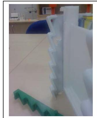
5. Insert the yellow sliding gel clamp into the hole closest to the core of the PAGE insert. Once inserted gently withdraw the sliding clamp outwards away from the core of the PAGE insert as shown.
