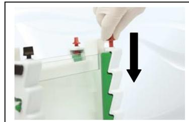
4. Continue to tighten the screw-pins until the gel clamps glide out of the resting slots and fix firmly against the glass plates pushing them upright.
