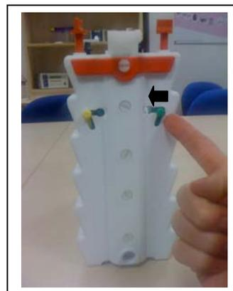
3. Push the green sliding gel clamp out of the PAGE insert by gently pressing the protruding pin as shown.
