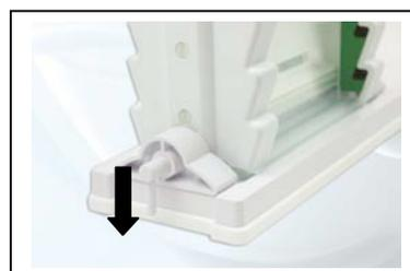
6. Insert cams and turn until tightened, drawing the PAGE insert onto the casting to form a leak-proof seal.
