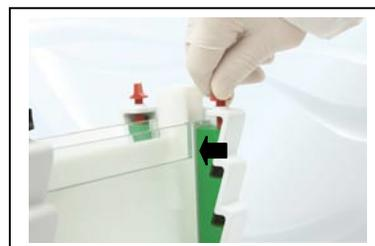
5. Check the bottom of the glass plates to ensure that they are flush together, and place the PAGE insert on the casting base; make sure that the cams are facing downwards.
