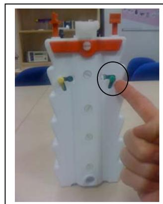
2. Gently push the green sliding clamp horizontally towards the core of PAGE insert until it can move no further.
