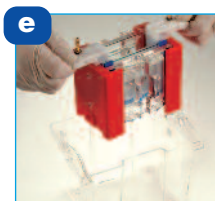
e Transfer to tank and fill with buffer
